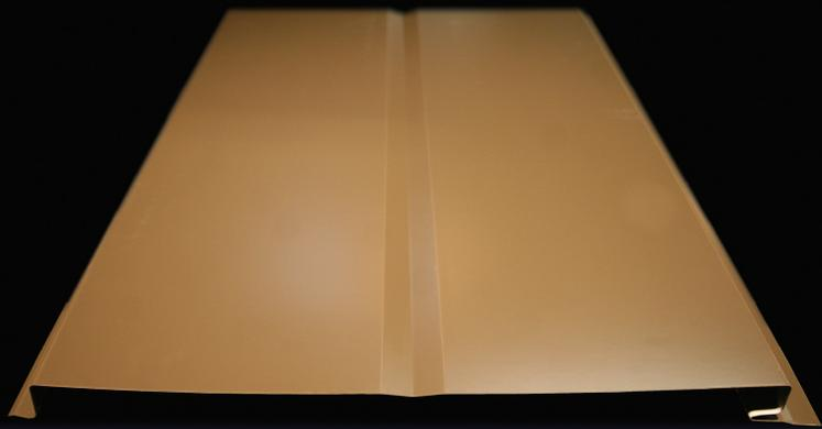
The SWP-12 Soffit-Wall panel is available in smooth and formed surface profiles, flush or reveal at 12" width, 24 gage Grade 50 Galvalume®. SWP-12 is a flexible product to meet every architectural design requirement calling for smooth or perforated panels. Architects choose which product will best meet their needs. The flexibility of our Soffit-Wall panel is that it allows for vertical and horizontal open framing or solid substrate installation. Priced to compete, proven to perform.
